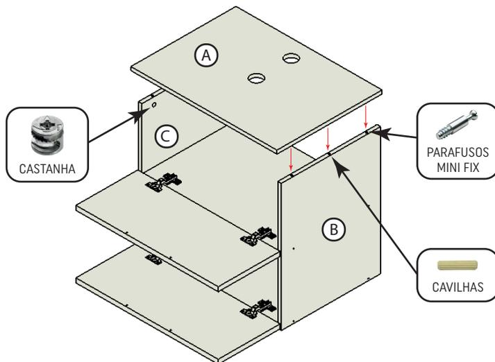
6. Parafuse as cantoneiras na parte interna traseira das Laterais (B e C) com os parafusos 4,0 x 12 mm.
